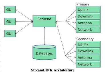
driven and require no modification to change from spacecraft to spacecraft. The specific communication protocol is implemented in a very modular fashion, limiting the impact and development time/cost of supporting additional missions.
