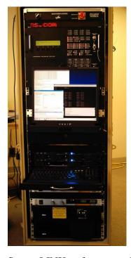
The Integrated Test Rack (ITR) is a complete EGSE test suite for command and control of spacecraft and other complicated systems. The ITR is a turn-key integration and test solution with capabilities proven through rigorous spacecraft I&T campaigns. Tiger Innovations EGSE racks have been used on the HENEX program, STPSat-1 mission, and are currently being built to support the STP-SIV mission with delivery in Fall 2007.
